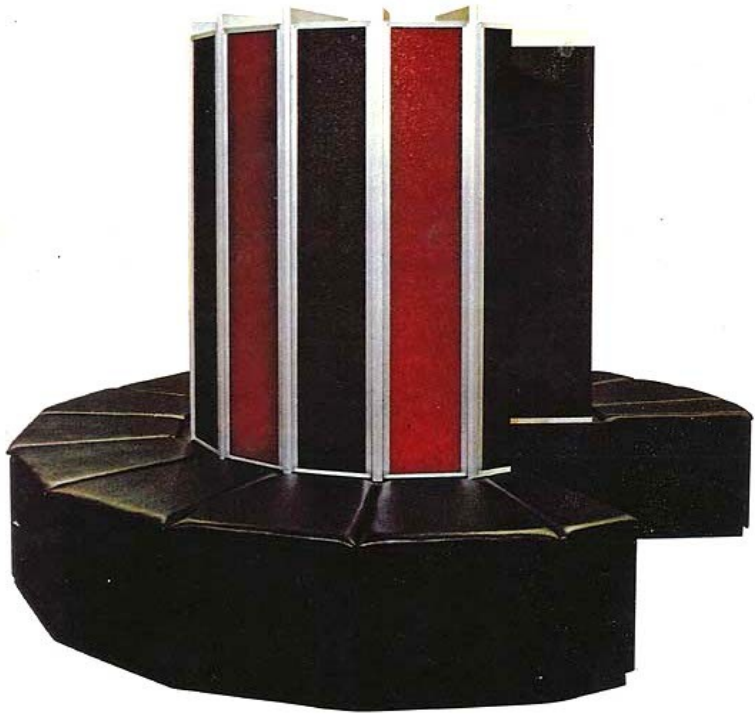
The Cray 1, early vector processor and universal icon of supercomputing. (Thanks, Cray 1 Hardware Manual Cover)
